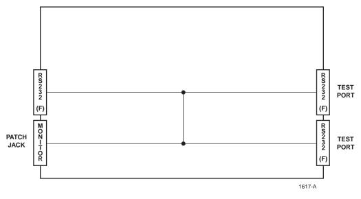
Figure 2-12. PSM-13 Test Module without LED Monitoring
